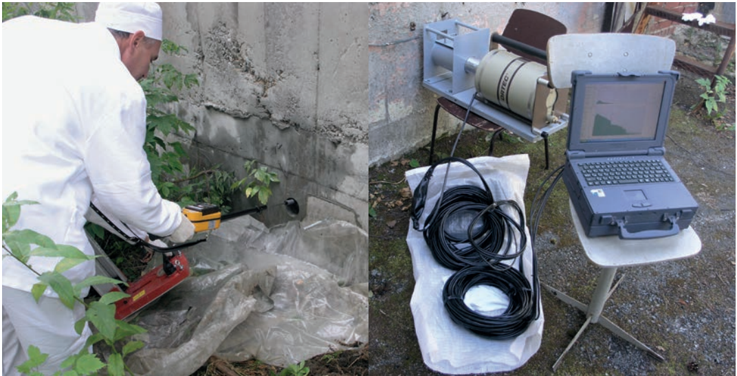
Portable measuring equipment for gamma analysis of contaminated structures (images courtesy PDC UGR)
