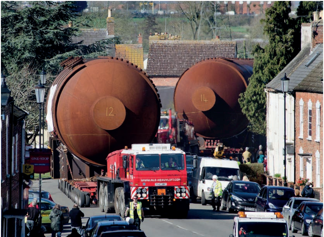
Boilers removed from the Berkeley site in the UK's Gloucestershire as part of the Magnox decommissioning programme. Fifteen 300 tonne boilers were taken to be recycled at Studsvik's metal treatment and recycling facility (now Cyclife) in Sweden (image courtesy Magnox Limited)
