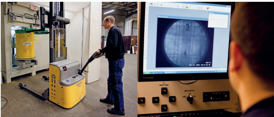
X-ray examination of waste drum (images courtesy SVAFO)
