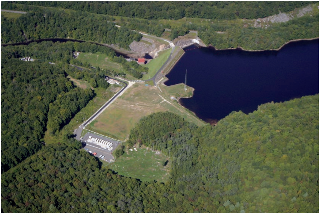
An interim spent fuel storage installation remains on the Yankee Rowe site, with 15 dry storage casks containing 533 spent nuclear fuel assemblies and one cask containing sections of the reactor vessel internals (image courtesy Yankee Atomic Electric Company)
