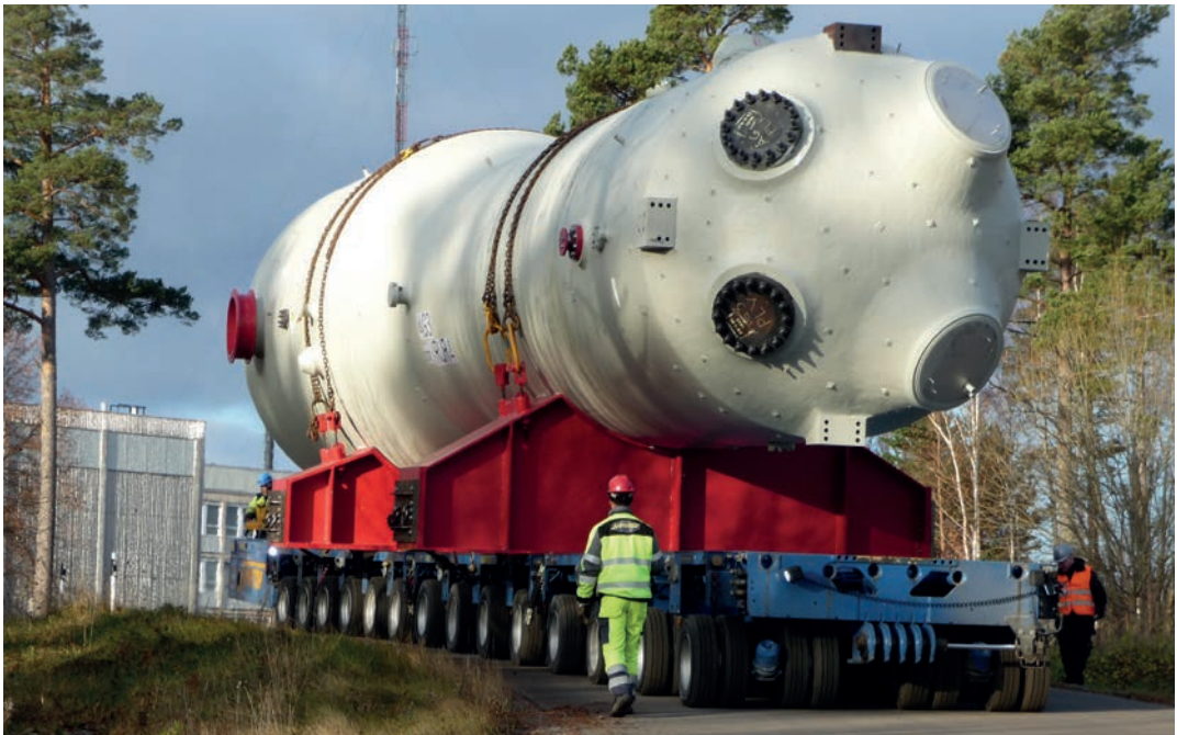
Ringhals 4 steam generator being transported to external treatment facility (image courtesy EDF/Cyclife)
