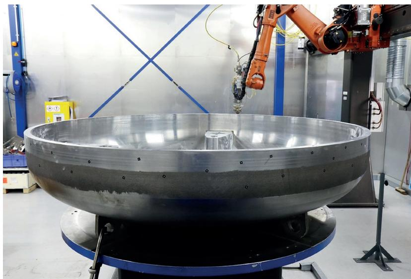
Figure 2. Diode laser cladding processing of a pressure vessel lower dome (NAMRC)
