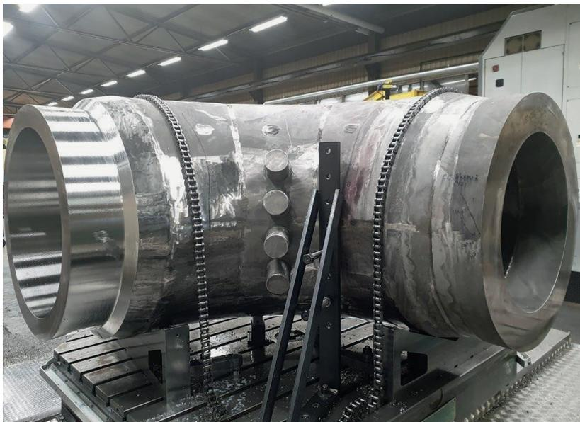
Figure 5. Piping elbow manufactured using HIP process (EDF/Framatome)
